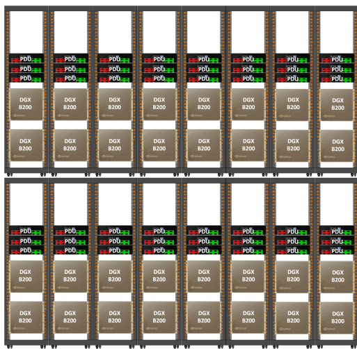
Figure 5.5 · A rack-scale reference point: a single scalable unit makes accelerator density, power distribution and cooling planning physical design inputs. Source: NVIDIA, DGX SuperPOD Reference Architecture, Figure 2. https://docs.nvidia.com/dgx-superpod/reference-architecture-scalable-infrastructure-b200/latest/dgx-superpod-architecture.html
